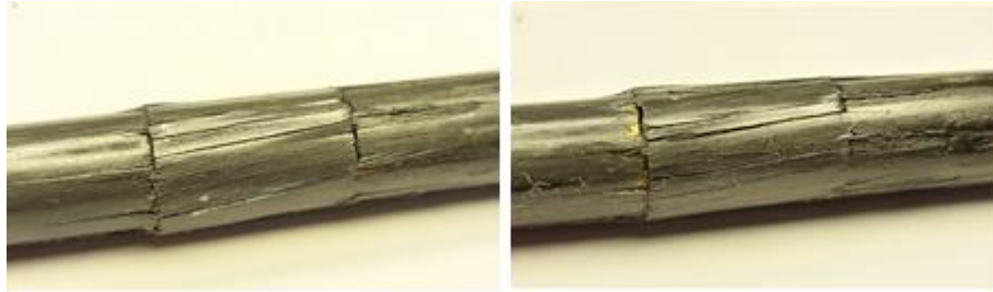
Figure 3: Carbon/epoxy fibre subjected to static torsion
